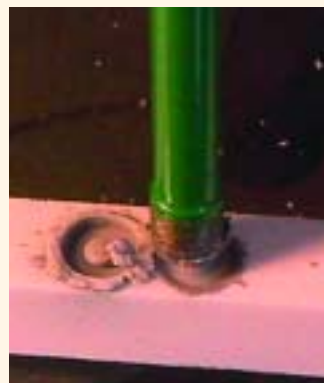
Drilling into an Al_2O_3 stick re-exposes diamonds after dressing.
